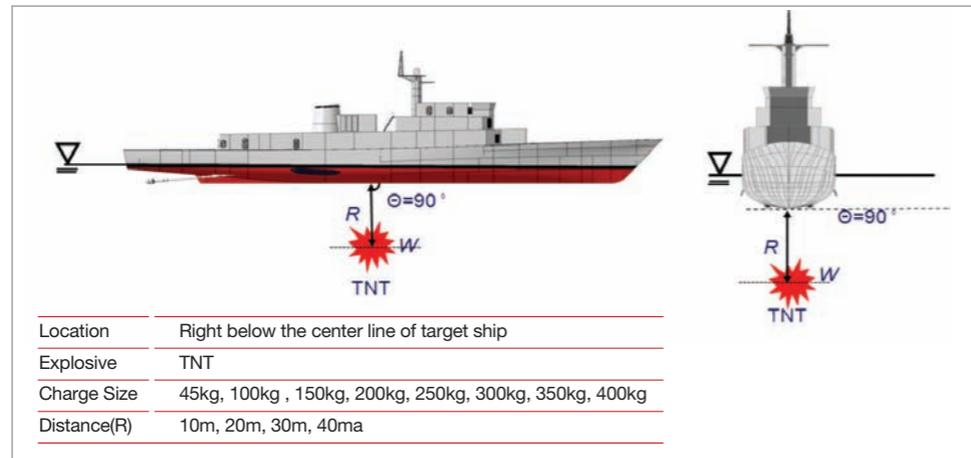
〈Figure III-6-1〉 Underwater explosion conditions for whipping analysis
