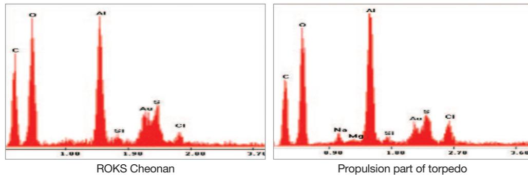
〈Figure III-5-11〉 EDS analysis result of adhered materials
