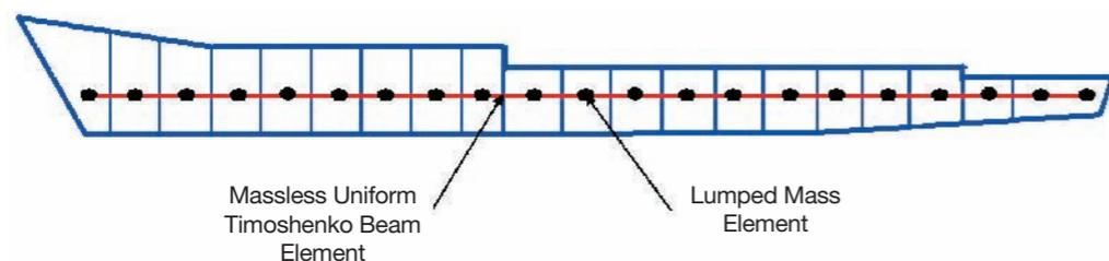
〈Figure III-6-2〉 Beam whipping analysis model
