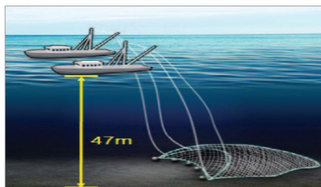
〈Figure III-8-1〉 Conceptual diagram of the special net and bull trawler
