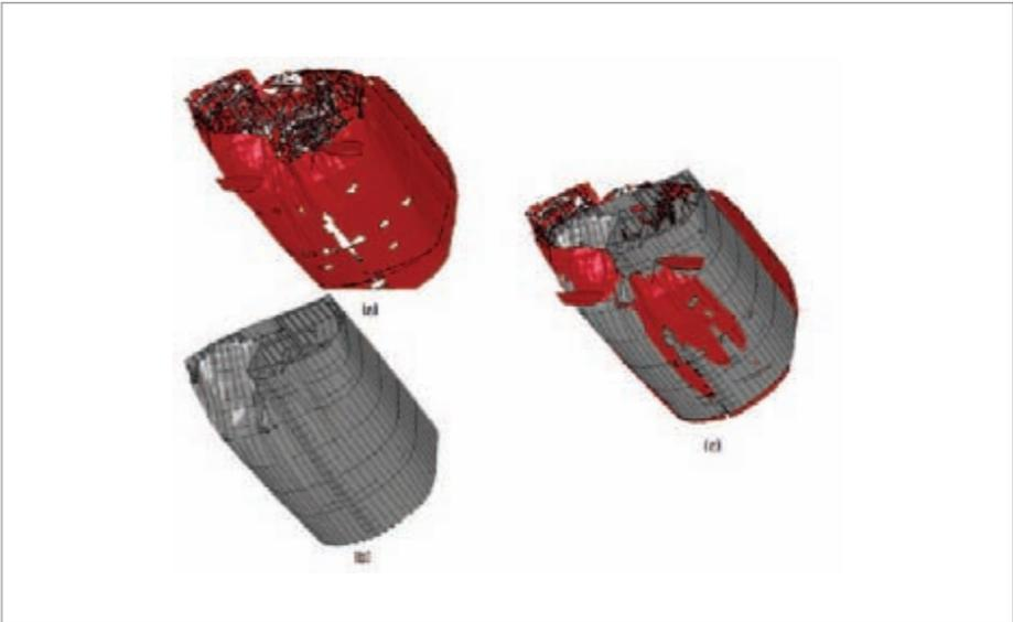
〈Figure III-6-25〉 Comparison between modelled damage and actual damage of ROKS Cheonan (bottom view of bow)
