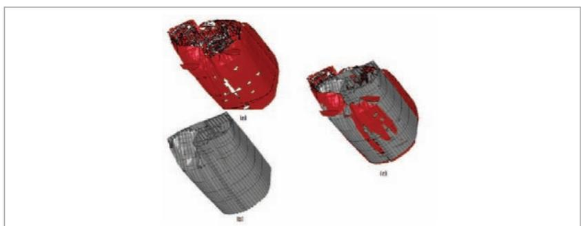
〈Figure III-6-28〉 Comparison between modelled damage and actual damage of ROKS Cheonan (bottom view of stern)
