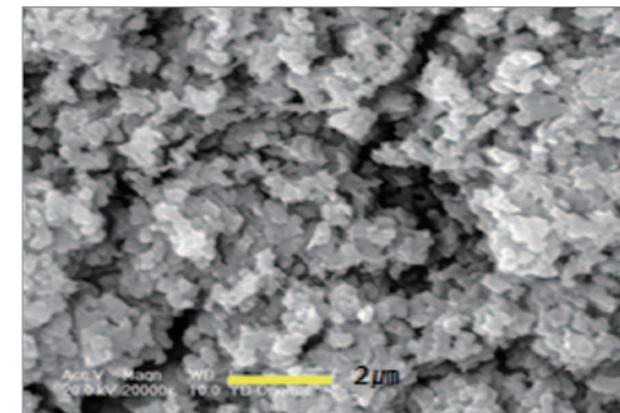
〈Figure III-5-10〉 SEM image of adhered materials
