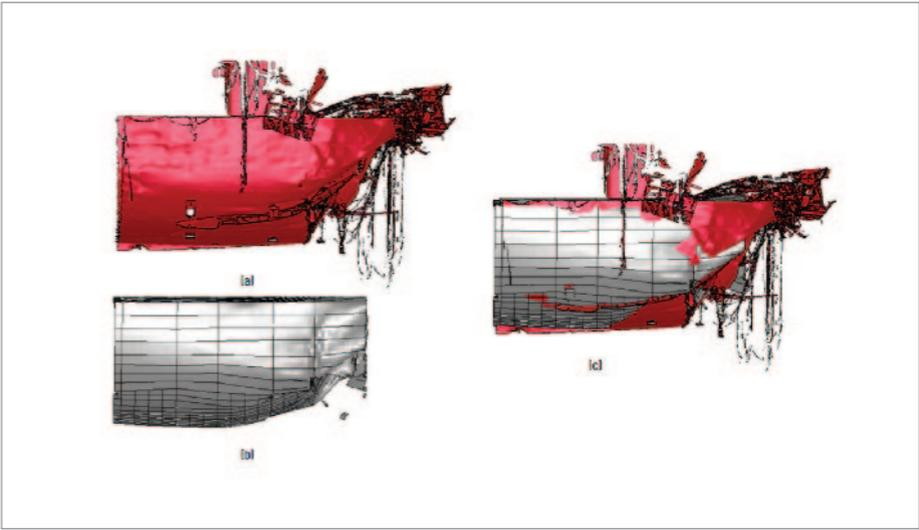
〈Figure III-6-26〉 Comparison between modelled damage and actual damage of ROKS Cheonan (side view of stern)
