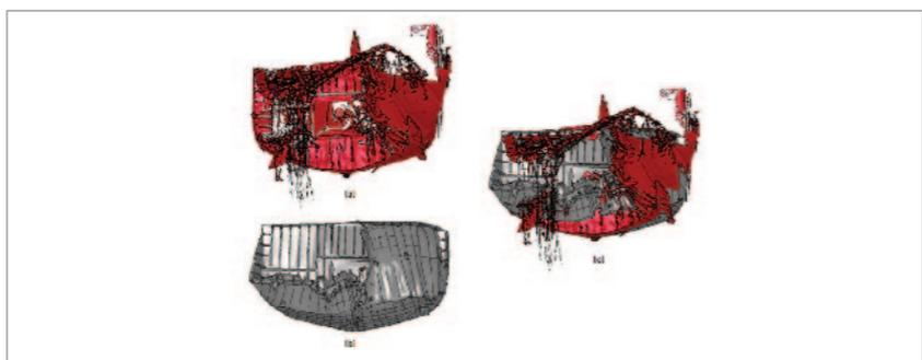
〈Figure III-6-27〉 Comparison between modelled damage and actual damage of ROKS Cheonan (front view of stern)
