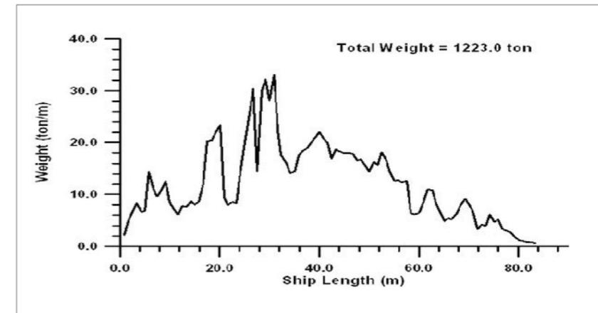
〈Figure III-6-3〉 Weight distribution along the ship in fully-loaded condition
