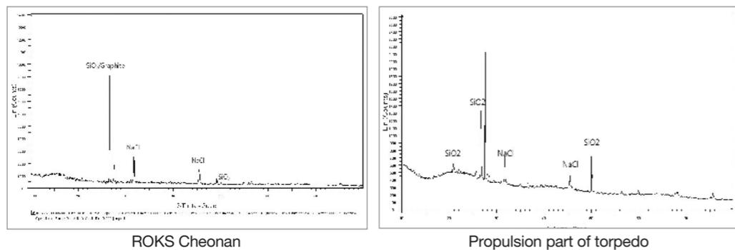
〈Figure III-5-12〉 XRD analysis result of adhered materials
