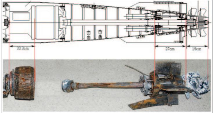
〈Figure III-8-5〉 Size comparison between the blueprint of CHT-02D and the evidence
