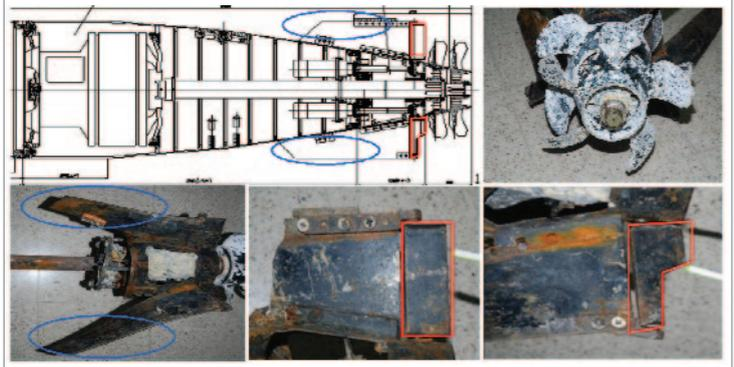
〈Figure III-8-6〉 Shape comparison between the blueprint of CHT-02D and the evidence
