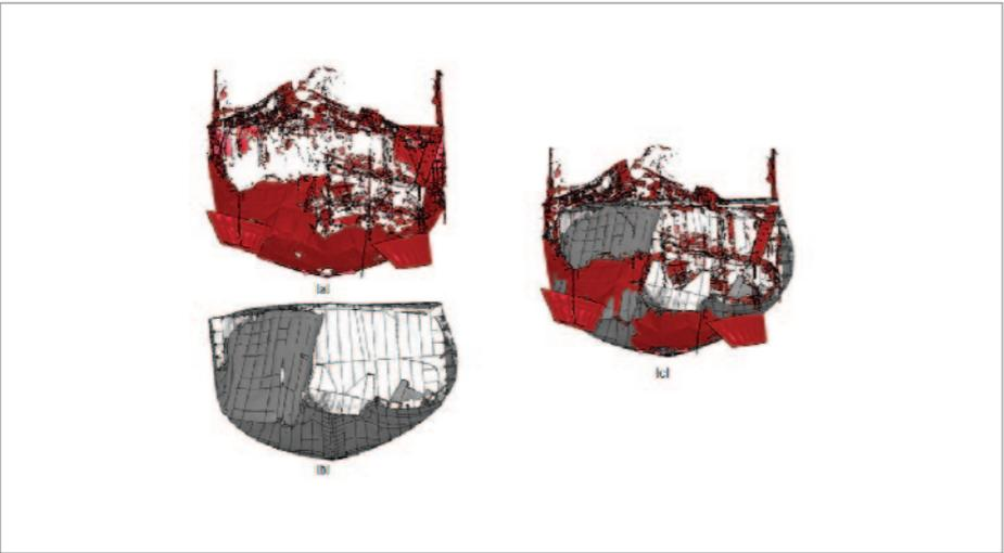
〈Figure III-6-24〉 Comparison between modelled damage and actual damage of ROKS Cheonan (front view of bow)
