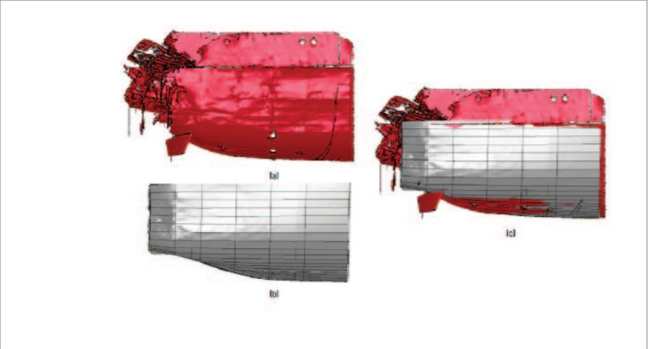
〈Figure III-6-23〉 Comparison between modelled damage and actual damage of ROKS Cheonan (side view of bow)
